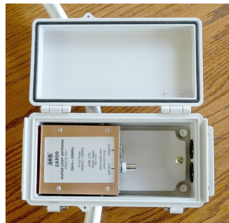
AOR LA800 Active Antenna ABS Plastic Box with Top Element Circuitry
